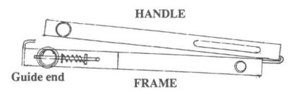
Pull hose guide away from frame and turn one quarter turn so guide is in the vertical position and locked in place with guide bars facing up.
