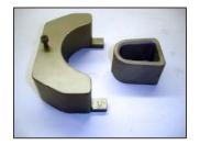
bend. The optional 90 degree bending shoe and collar make it simple to repeat 90 degree bends without a guide. The optional bending collar increases the bending radius and minimizes rebar breakage especially on #5 grade 60 rebar. This portable electric/ hydraulic rebar bender comes complete with a steel carrying case, hydraulic oil & tool kit. Benner-Nawman backs it with a one-year warranty.
